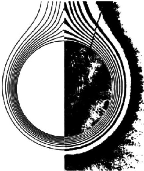
Fig. 3. Calculated temperature contours (left hand side) and the experimental fringe pattern (right hand side, Kuehn and Goldstein [6]) around horizontal circular cylinder at Ra = 10^5 .
